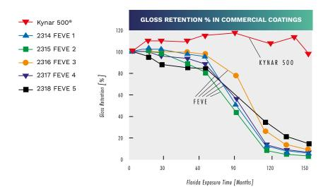
In typical formulations (see shaded areas), Kynar 500° resin-based coatings contain higher fluorine levels than FEVE-based coatings, resulting in greater resiliency, color and gloss retention.
