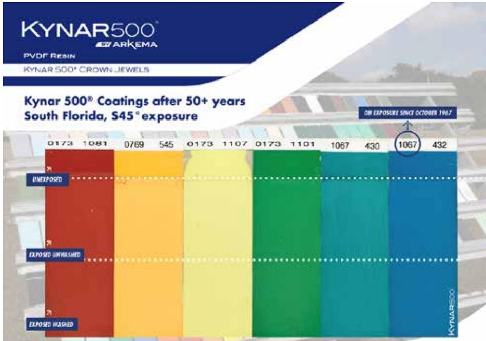
compiled by an independent, accredited testing laboratory and are based on actual exposure time in Southern Florida as required by high performance, organic coating specifications AAMA 2605.
